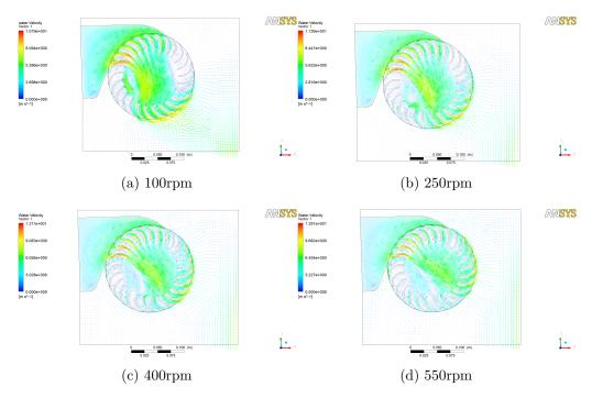
Figure 5.9: Prototype B velocity vectors variation with rotational speed
