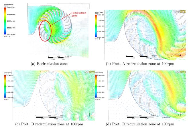
Figure 5.16: Some prototypes recirculation zone
