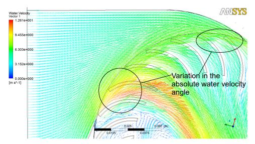
Figure 5.7: Water absolute velocity vector in the nozzle outlet
