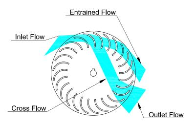
Figure 2.3: Runner with Cross Flow and Entrained Flow Behavior
