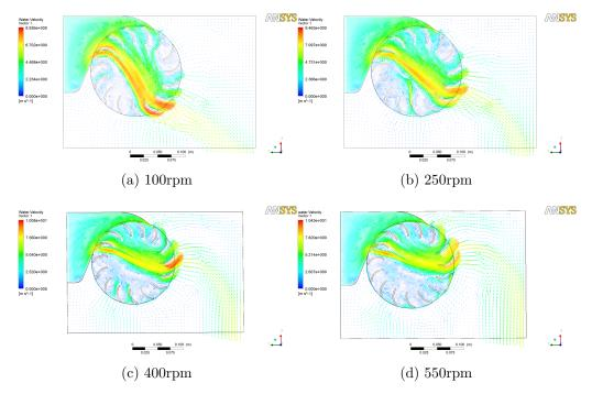
Figure 5.10: Prototype C velocity vectors variation with rotational speed
