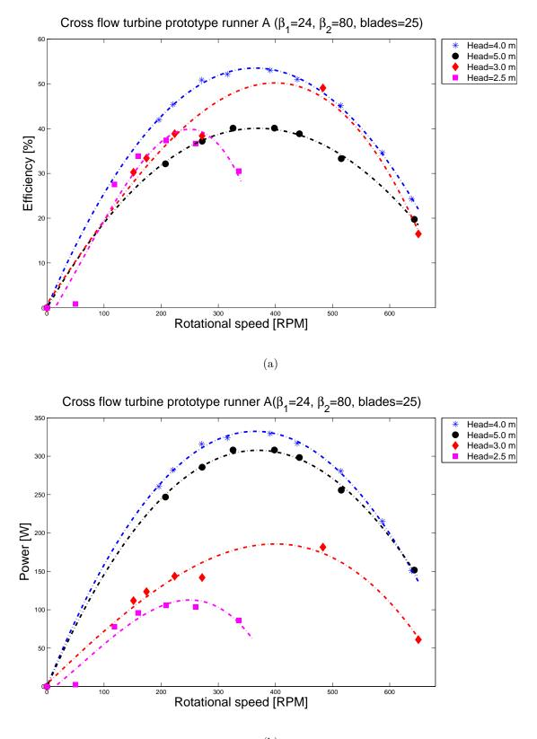
(b) Figure 5.1: Characteristic curves of A
