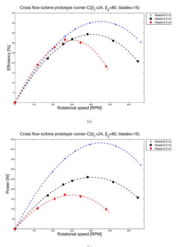
(b) Figure 5.3: Characteristic curves of C
