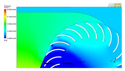
Figure 5.21: Pressure located at the nozzle outlet and runner inlet
