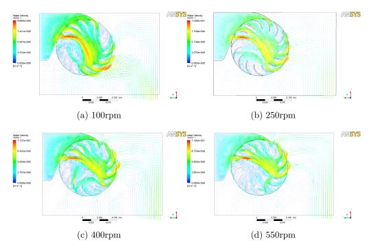
Figure 5.11: Prototype D velocity vectors variation with rotational speed
