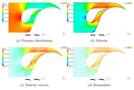
Figure 5.24: Nozzle with inner guide vane CFD results
