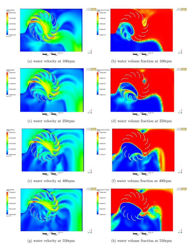
Figure 5.15: Prototype D velocity and volume fraction variation with rotational speed
