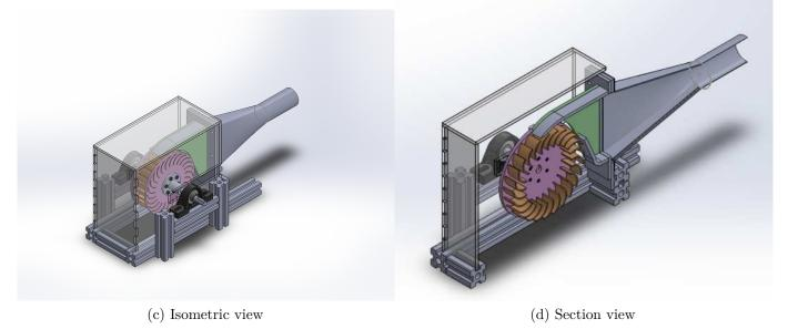
Figure 3.1: Cross flow turbine prototypes 3D Model
