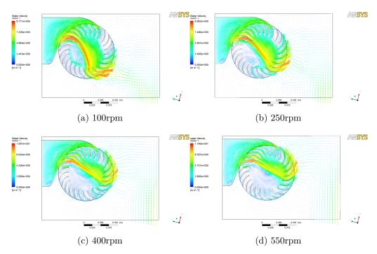
Figure 5.8: Prototype A velocity vectors variation with rotational speed
