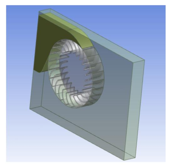
Figure 4.2: Assembly of the turbine CAD model in DesignModeler
