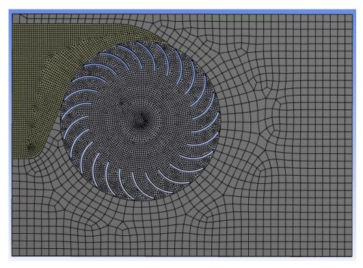
Figure 4.3: Turbine mesh
