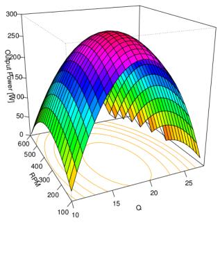
Power Response Surface Flow Rate [Lps] vs Rotational Speed [RPM]
