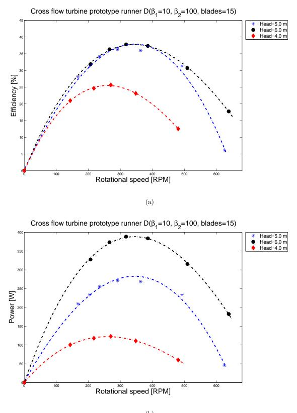
(b) Figure 5.4: Characteristic curves of D
