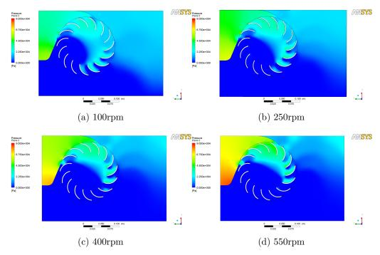
Figure 5.20: Prototype D pressure variation with rotational speed
