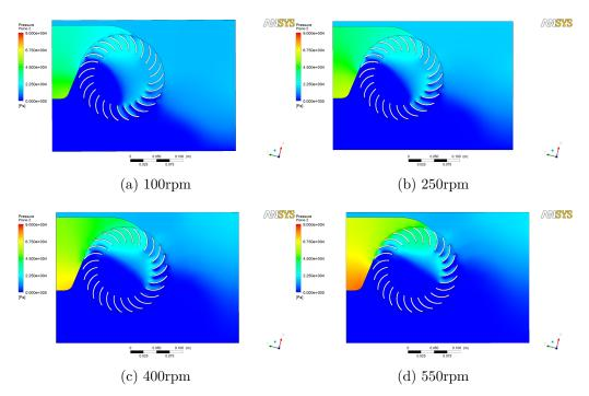
Figure 5.17: Prototype A pressure variation with rotational speed
