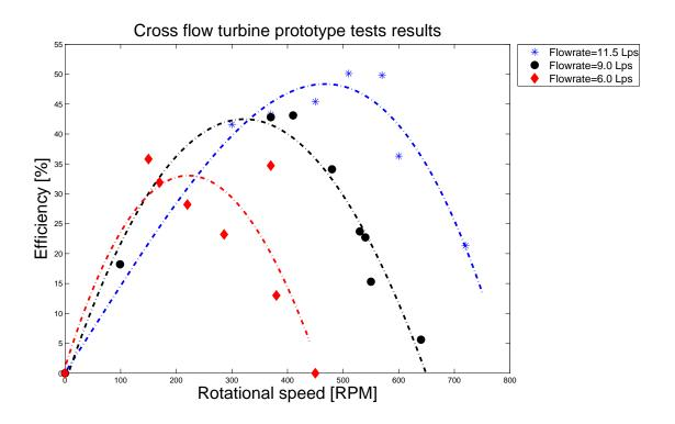
(a) Efficiency Vs. Rotational Speed
