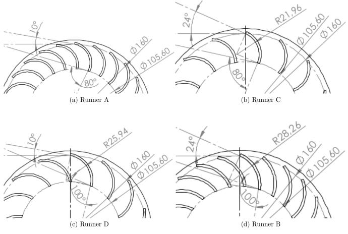
Figure 3.3: Blade geometry
