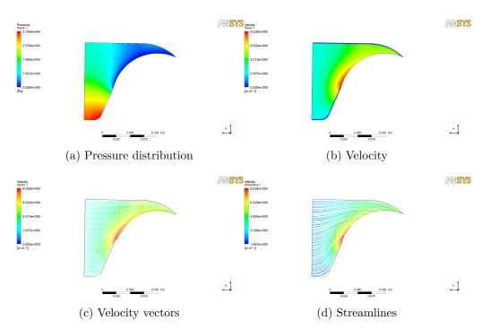
Figure 5.23: Nozzle without inner guide vane CFD results
