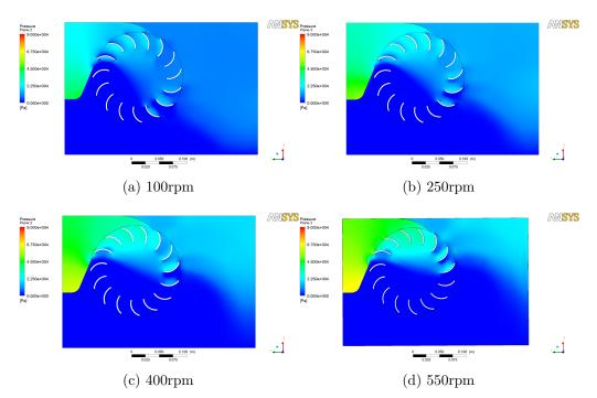
Figure 5.19: Prototype C pressure variation with rotational speed
