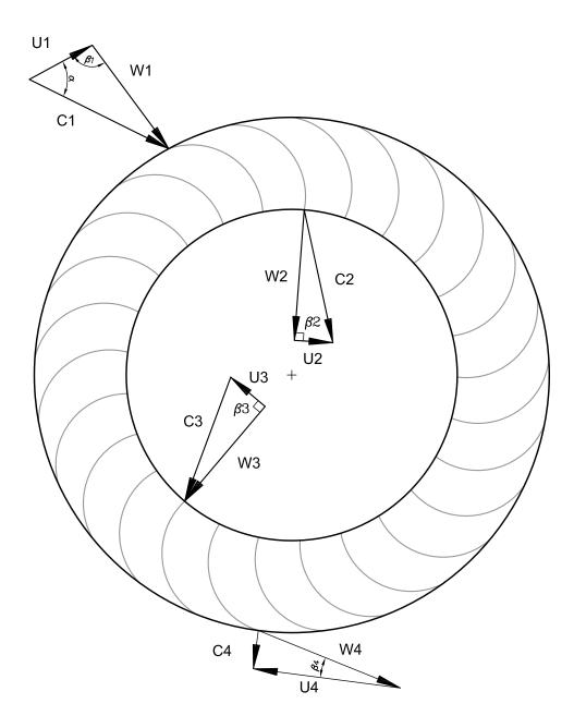
Figure 2.4: Velocity Triangles of a Cross Flow Turbine
