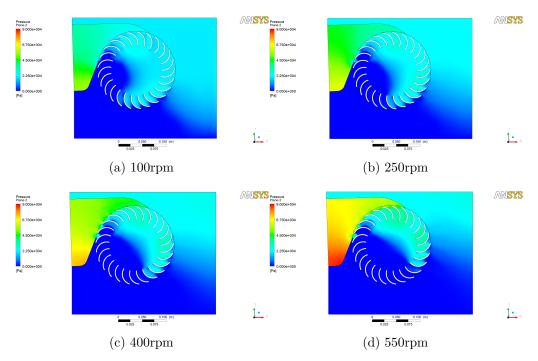
Figure 5.18: Prototype B pressure variation with rotational speed
