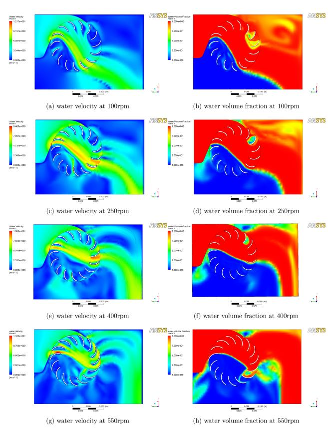
Figure 5.14: Prototype C velocity and volume fraction variation with rotational speed
