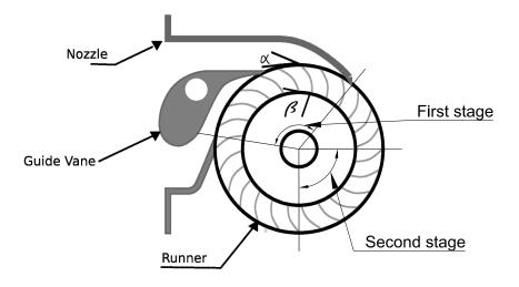
Figure 2.1: Definition sketch of the Cross Flow Turbine
