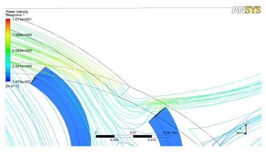
Figure 5.22: Entrained flow detected in CFD analysis
