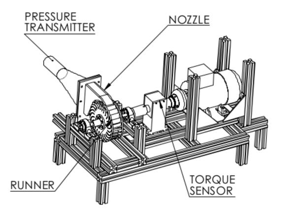
Figure 3.5: Test bench used for experiments
